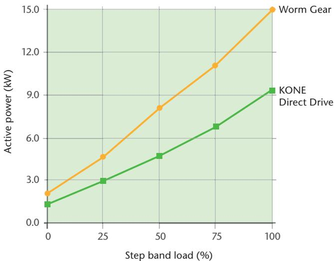
Energy measurements made at a Helsinki Metro station on November 23<sup>rd</sup>, 2011.
